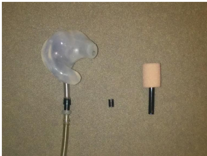
Figure 3. Coupling the child's earmold to the ER-3A can be more securely achieved by cutting the black insert tubing which can be used to connect the earmold to the earphone tubing.
